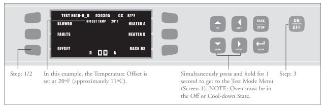
FIGURE 29: Adjusting the Temperature Offset
